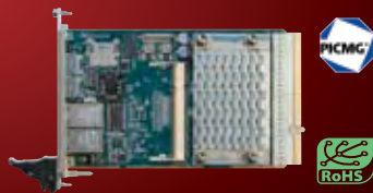
A3pci7512 *Freescale MPC7447A (1GHz)
